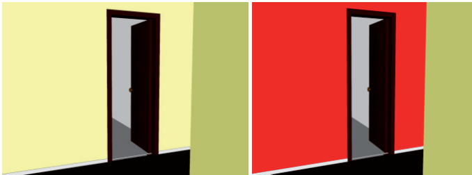
Figure 18. Chromatic alteration of the coating according to its state of deterioration.
