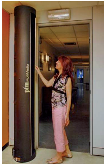
Figure 9. The compact hardware of the HoloMachine. The woman indicates the slots from which the micro-particles of water are ejected. Courtesy of PFM Multimedia (Milan, Italy)
