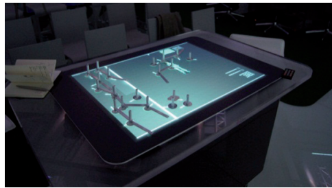
Figure 12. The Surface Table with tangible CMA (Ceiling Mounted Arm) systems used for the operating theater design case study.
