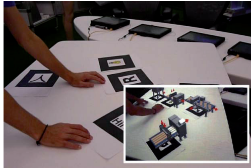
Figure 15. The Augmented Reality Table. The picture shows the markers and (inset) the virtual models projected on top of these markers.
