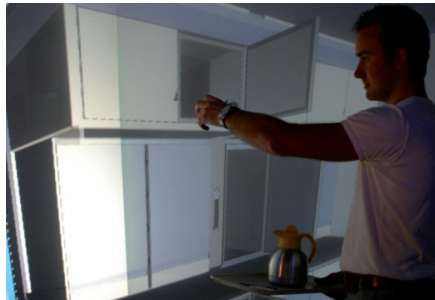
Figure 5. The virtual aircraft galley allows users to interact with the virtual model.
