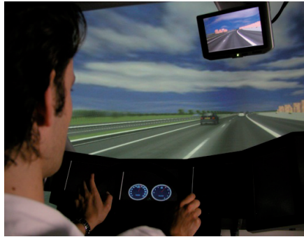
Figure 2. The driving simulator used for testing lane-change support systems, also showing the configurable dashboard.
