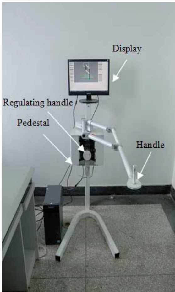
Figure 4. Upper limb rehabilitation robot based on magnetic powder brakes
