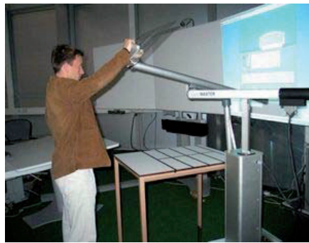
Figure 11. A designer testing the haptic lid emulator. The display on the right shows a digital representation of the machine that is linked to the haptic device.
