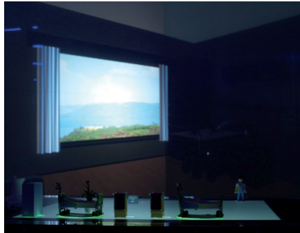
Figure 3. The room layout configurator. The foreground shows the surface table with tangible objects. The background shows the wall display with the virtual room.
